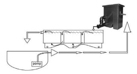
As a mechanical pre-filter for existing trickle filter systems (C).
