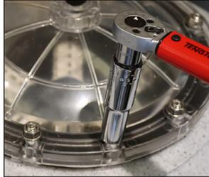
Carefully undo all 12 nuts (M8) using a torque wrench and remove washers. Keep them safe.
