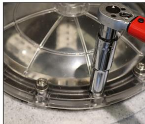
Use a torque wrench pre-set at 9Nm until clicks following the tightening sequence.
