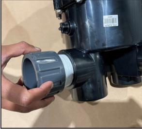
Screw the threaded connector into the multiport valve.
