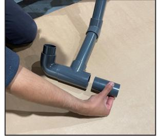
Push in the other 9cm pipe into the t-piece on the pipework assembly. **YOU WILL GLUE THIS CONNECTION LATER.**
