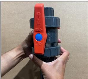
If the blower ball valve is not connected, screw the union onto the ball valve. **HAND TIGHTEN ONLY.**
