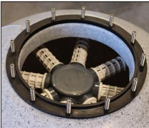
Ensure the large, black O-ring around the lid is in place. Gently push it down before re-fitting the lid.
