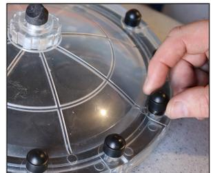
Re-fit the 12 plastic caps over the top of the nuts. Ensure the air relief bleed valve is screwed into the lid.
