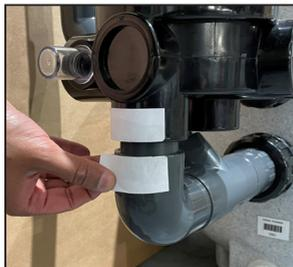
Apply two pieces of masking tape flush to the points where the multiport valve outlet and the connecting pipe join.
