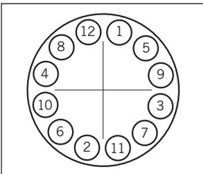
**YOU MUST** follow the 12 Bolt Torque Pattern sequence when tightening the nuts.
