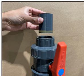
Take the 6cm pipe insert. At one end, clean and glue the outside of the pipe and the inside of the ball valve and push together.
