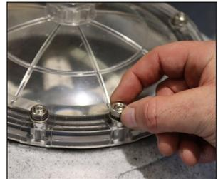
Re-fit all 12 x M8 washers onto studs and the M8 nuts.
