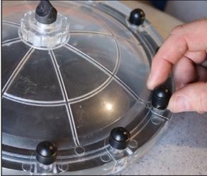
Remove the 12 plastic caps covering the nuts on the lid collar. You may need to use a flat head screwdriver.
