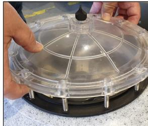
**TO RE-INSTALL** - Carefully place the lid over the studs.
