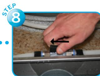
Open the air valve to the outer chamber.
