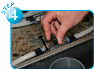
Close the valve to the outer chamber.
