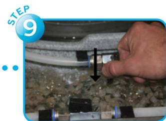
Close the air valve to the inner chamber.
